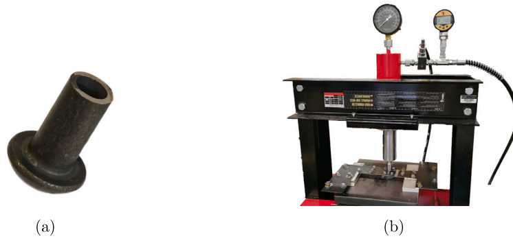
Fig. 10. Components of the riveting setup: (a) semi-tubular rivet (DIN 660B), (b) hydraulic riveting device with pressure sensor.
